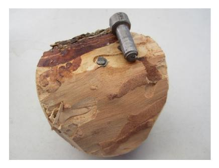
As you can see it's done for and the blank is a piece of well dried Eucalyptus and very hard. But on closer examination it looks like the screw was cracked for quite some time and it finally come apart. It fell off at low speed which was good.
