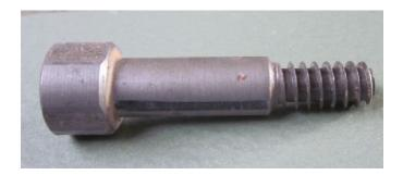
All I used was a hacksaw and a battery drill with a cross blade screw driver head fitted, now you can use an ordinary cross blade screw driver. But the blank has got a good hold on the screw and the drill will just make it easier and quicker to get out. I used an impact drill, but any drill with variable speed will do, it was the nearest drill at the time.
