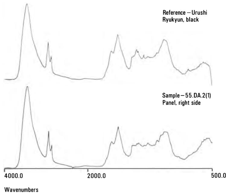
Figure 2. Infrared absorbance spectra of two urushi samples. The sample on top is from a Chinese black lacquered food bowl, and the sample on bottom is from the lid of a black lacquered bowl set thought to be of Japanese origin. This visual identification was concurred by computer matching.
