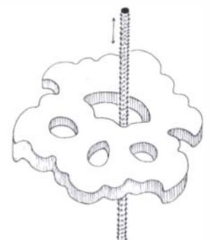
Figure 10. Raden from the Shigure kura (saddle; thirteenth century) showing the marks of a blade with a round cross section.
