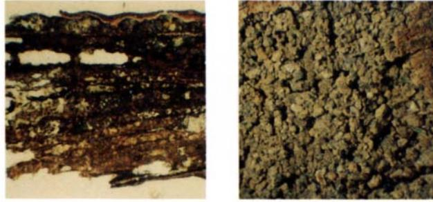
Figure 4. Urushi-shitaji used to bind cloth in a shippi-bako (leather box) from the Horyuji treasures.
