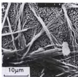
Figure 3. SEM photomicrograph of the fibrous polysaccharides.
